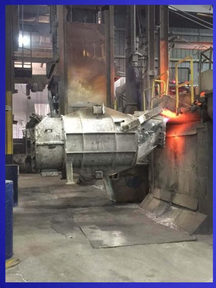
GF converter system with a pure Mg treatment.
